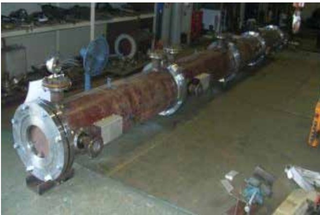
Heat Pipe Fabrication
